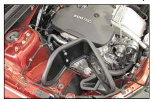
9. Install the heat shield assembly onto the engine mount and secure with the factory bolt from the previous step.
