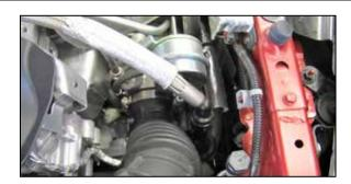
3. Disconnect the crank case vent hose.
