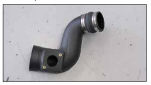
10. Install the provided hump coupler (084018) hose onto the K&N® intake tube and secure with the provided hose clamp.
