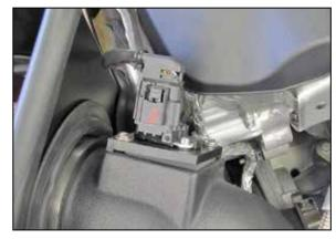
Reconnect the mass air sensor electrical connection.
